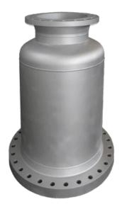
Pressure reduction in gas or steam networks is often achieved by control valves, frequently accompanied by high levels of noise generation. Pressure reduction over several stages also reduces the generated noise. Axces Steam and Flow Control have an excellent solution for this in the form of noise attenuating diffusers located immediately downstream from the control valve. This method of noise attenuation is compact, efficient and demands no maintenance.
